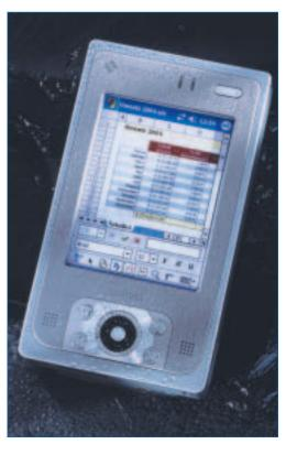
The IT-10 has been designed for maximum durability. It can withstand a drop from 1 meter onto concrete. Furthermore the IT-10 is dust and waterproof according to level IP54 (International Standard IEC60529). The internal components are sealed inside an extremely tough yet light magnesium inner shielding. The outer casing is made of durable plastic resin to give added protection. The LCD touch screen is set in a shock absorbent rubber mounting to resist the effects of hard impacts.
