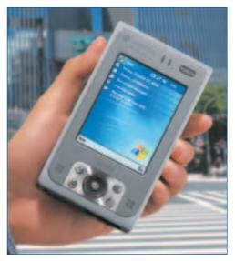
The IT-10 has a fine 3.7 inch transflective TFT color LCD which is capable of displaying full VGA resolution (640 x 480). This is 4 times the number of pixels of conventional QVGA screens and makes the IT-10 ideal for displaying web based applications which contain detailed images. The screen displays conventional QVGA applications without modification so you can continue to use software origi-
