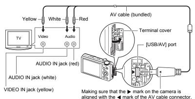
Make sure that you insert the cable connector into the USB/AV port until you
