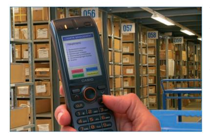
The DT-X7 works with Windows<sup>®</sup> CE<sup>®</sup> 5.0 and offers 64MB RAM working memory. Versatile, reliable standard software can be integrated as well as especially customized business solutions.
