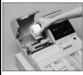
Ensuring the paper is being fed from the bottom of the
