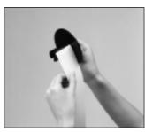
Slide the leading end of the paper into the groove on the spindle of the take-up reel and wind it onto the reel two or three turns.
