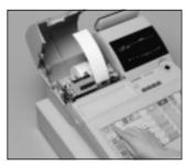
Press the key until about 20 cm to 30 cm of paper is fed from the printer.
