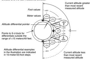
Altitude differential is indicated in the range of +15 meters, in 1-meter units. · Altitude is calculated and displayed using meters as the standard. Altitude can also be read in feet units as shown in the illustration
