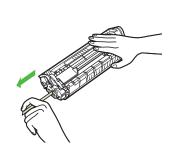
Pull out the seal completely.
