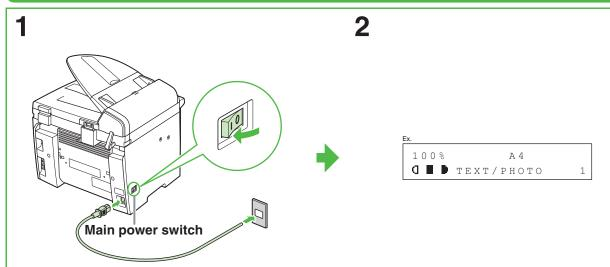
Connect the power cord into the rear socket and the wall outlet, and press the [I] side of the main power switch to ON.
