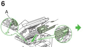
Align the guide (A) on the left side of the toner cartridge with the groove inside the machine.
