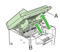
Lift the scanning platform until it is locked (A), and open the printer cover (B).
