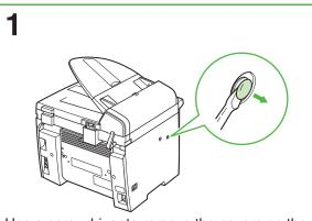
Use a screwdriver to remove the covers on the left side of the machine.
