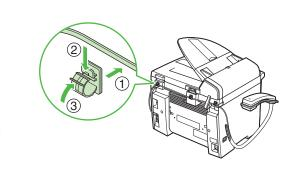
Attach the handset clamps to the back side of the machine, hook the handset cable on the clamps, and close the clamps.
