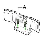
Insert the plugs with pins (A) into the holes on the handset cradle.
