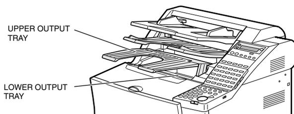
When the face-up tray is open, the fax will automatically select face-up delivery. To select face-down delivery, make sure the face-up tray is closed. If the extension of the face-up tray is extended, be sure to push it back into the tray before closing.
