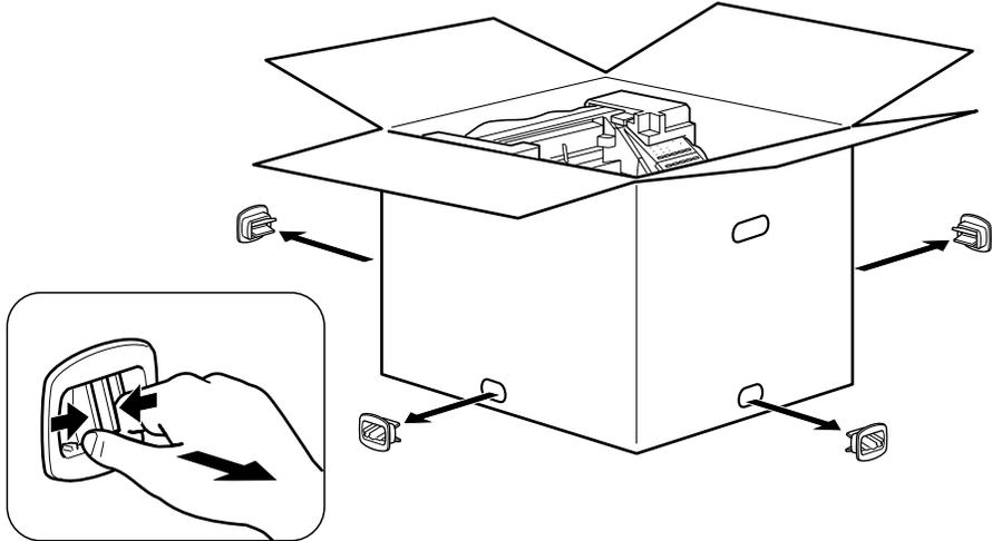
4. Lift and remove the upper carton. Remove the four styrene foam blocks positioned on top of the fax unit. Then lift the fax unit by gripping the handles on the right and left sides. (→2-10)
