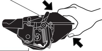
DO NOT TOUCH THE PROTECTIVE SHUTTER ON THE BOTTOM OF CARTRIDGE.
