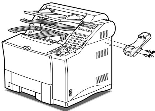
4. Connect the end of the handset connector cord to the extension phone jack marked with the handset icon (
