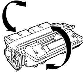
4. Place the new cartridge on a stable, flat, clean surface, and snap the tab to detach it from the cartridge.
