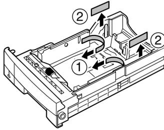
5. If a spacer is attached, remove it from the paper cassette while pressing the bottom plate.
