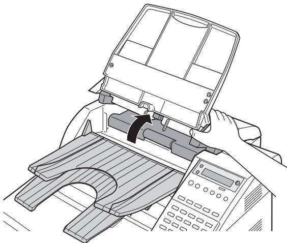
7. While holding the ADF cover open with one hand, use one finger of your other hand to gently push in the black plastic loop to separate it from the stub on the fax machine.
