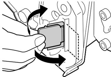
5. As you steady the cartridge with one hand, remove the seal by gently pulling the plastic tab with your other hand. Use a firm, even pull to avoid breaking the seal.
