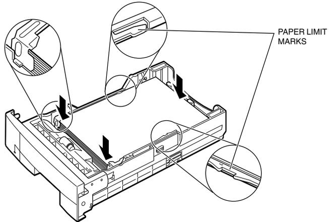
6. Press the paper stack down to make sure it has a clearance of approximately 0.04 in. (1 mm) from the hook of the paper size rear guide.
