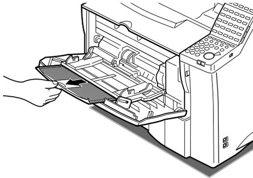
3. The MP tray holds approximately 100 sheets of paper. Before you load paper on the MP tray, tap the edges of the stack to make sure the leading edge and sides of the stack are even.
