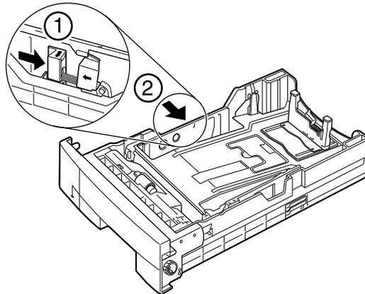
Push up the stopper of the paper size rear guide, and slide it to the mark indicating the desired paper size.
