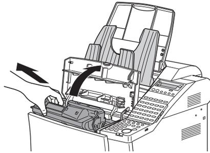
3. While holding the green lever, flip the transfer guide up. Gently ease the edge of the paper away from the guide. After the paper rear-most edge has come out, slowly pull the paper forward and out of the fax unit.
