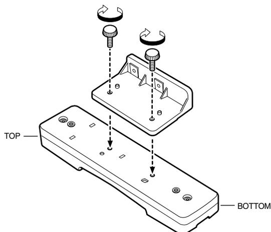
2. Fit the handset cradle holder over the holes on the fax unit.
