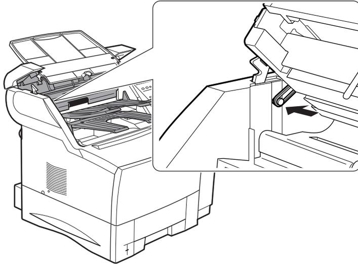
12. Close the ADF cover and press down on it slightly until you hear it lock in place, and lower the document feeder tray.
