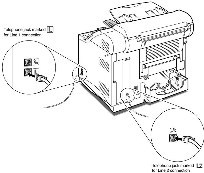
4. Connect the other end of the two telephone lines to the wall telephone jacks.
