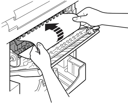
3. After the paper's edge has rolled out, pull the paper forward carefully.
