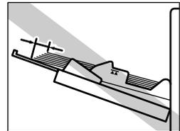
1. Pull the MP tray out using the handle on the panel.
