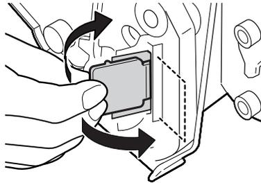
7. As you steady the cartridge with one hand, remove the seal by gently pulling the plastic tab with your other hand.
