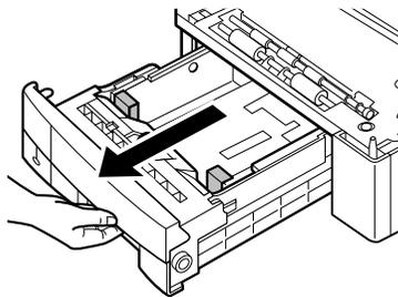
3. If tapes are attached to the paper cassette, remove them. Then remove the spacers under the paper guide clips by first pressing down on the bottom metal plate with one hand and then sliding the white spacers inwards with the other hand.
