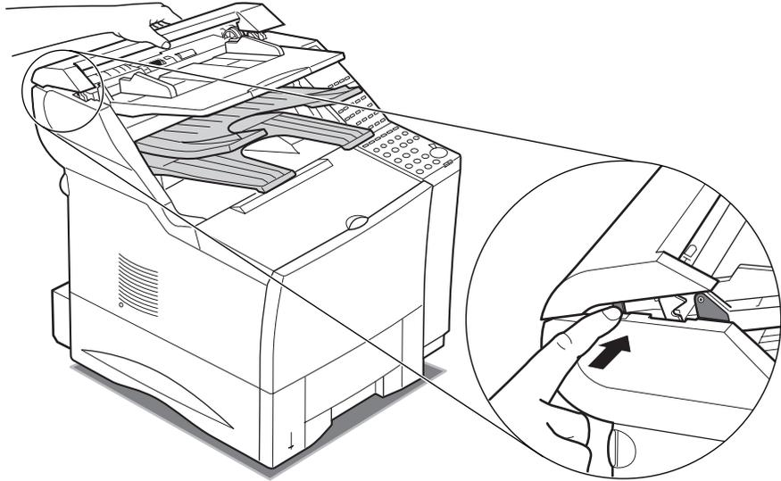
4. Open the upper unit of the ADF cover fully and clean the rollers.
