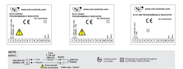
Note: 1) Mains supply cords shall meet the requirements of IEC 60227 or IEC 60245. 2) In accordance with the safety regulations, the power supply switch shall bring the identification of the relevant instrument and it should be easily accessible by the operator.
