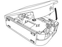
• Make sure that the end of the tape feeds under the tape
