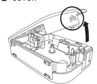
Verify that the P-touch labeler is turned off. Open the cassette cover as shown by the arrow in the above illustration while pressing the part marked "<<".
