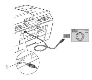
Turn on the camera. When the machine has recognized the camera, the LCD shows Camera Connected.
