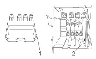
If you are not able to find the orange protective part, DO NOT remove the ink cartridges before shipping. It is essential that the machine be shipped with either the orange protective part or the ink cartridges in position. Shipping without them will cause damage to your machine and may void your warranty. 9 Wrap the machine in the bag.
