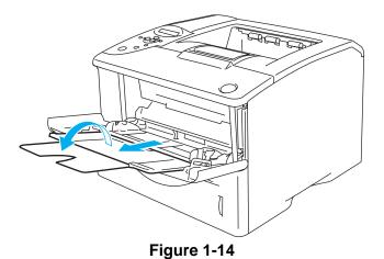
**4** Put paper in the MP tray. Put the side to be printed on first, face up, with the leading edge (top) of the paper in first. Make sure the paper touches the back of the tray and remains under the maximum paper height guides on both sides of the tray. Do not put more than 100 sheets of paper (80 g/m² or 20 lb) in the MP tray at any one time, or it may cause a jam.
