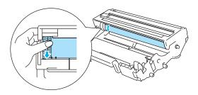
When you have located the mark on the drum that matches the print sample, wipe the surface of the OPC drum with a cotton swab until the dust or paper powder on the surface comes off.
