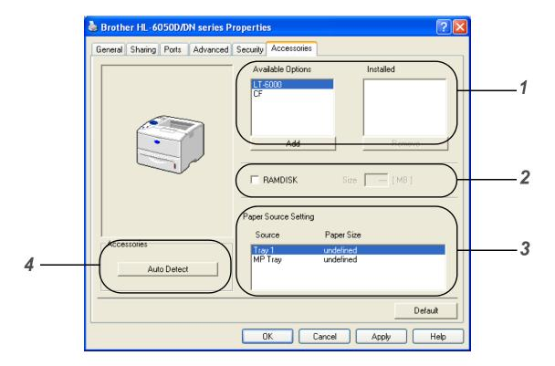
1 You can manually add and remove the options for any optional unit device that is installed on the printer. Tray settings will match the installed options.
