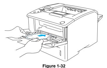
Make sure that the envelopes are neatly stacked and in the proper position in the MP tray. If they are not, the envelopes may not be fed properly, resulting in a skewed printout or a jam.
