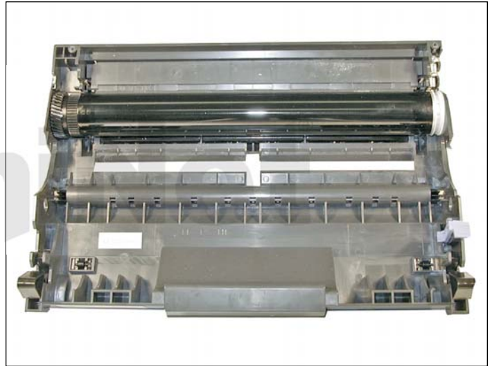
14. Install the drum and associated gear, hub, and spring.
