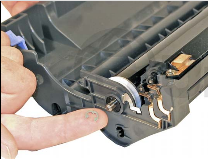
3. Remove the E-ring from the non-gear side of the drum axle shaft.
