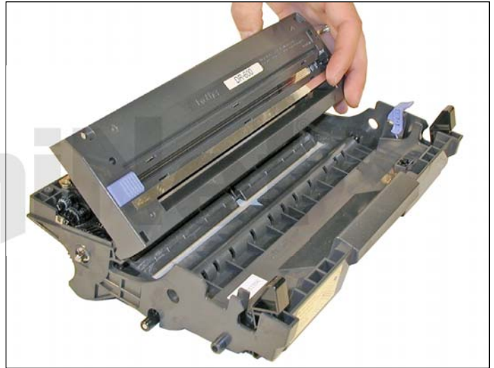
2. Lift the top cover up towards the empty toner cartridge cavity and remove from the cartridge.
