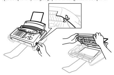
**2** Remove the print cartridge containing the used ribbon and set it upside—down with the blue gear in the upper left corner.
