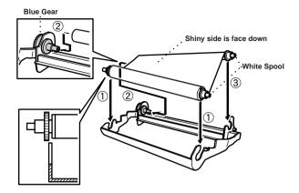
**7** Turn the upper right white spool *clockwise* to tighten the ribbon, as shown.
