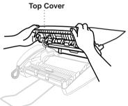
**3** Pull the jammed printout gently from the paper tray toward the *front* of the machine. If the printout is jammed, then pull it toward the *back* of the machine.
