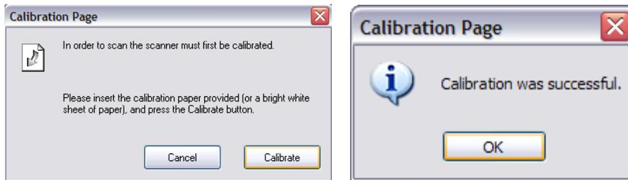
This calibration process uses the special black and white calibration sheet (see picture on page iv) that was included with your scanner (Visit <http://www.brothermobilesolutions.com> to order additional calibration sheets and cleaning kits). When calibrating, make sure the side with the black bar is facing down and note the direction of the arrows for proper insertion.
