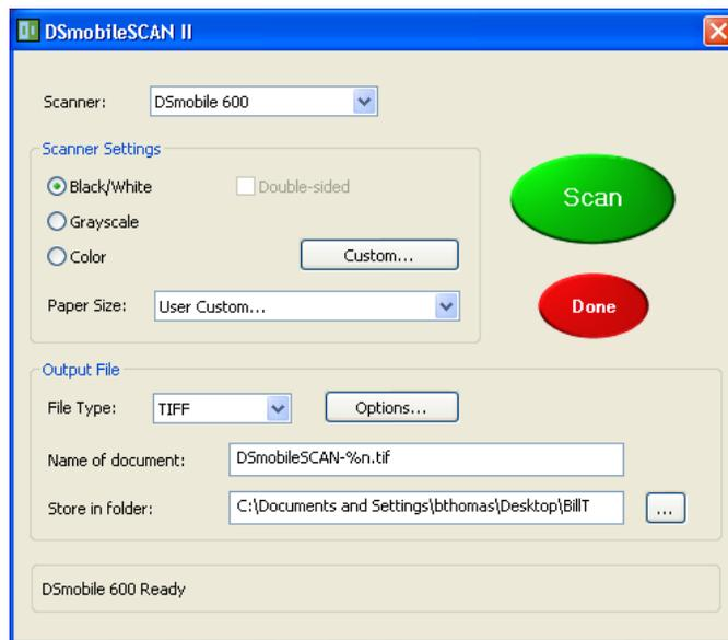
This program gives the user the choice of selecting type of scan and paper size from the main menu (shown above) or pressing the “Custom” button to utilize the document manager control panel for more precise settings. Selecting the custom settings will put the program into a TWAIN driver (as defined on page 16) and takes you out of the actual DSmobileSCAN II software application.
