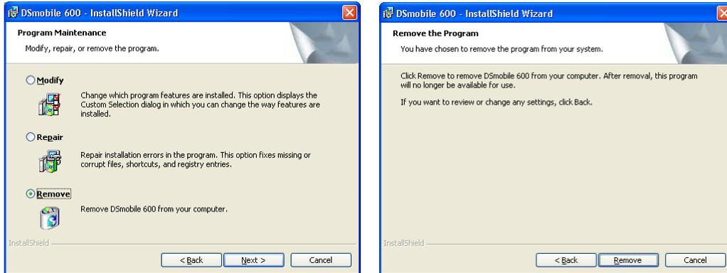
If you should need to un-install Windows scanning software (DSmobileSCAN II or PageManager), select Start, Control Panel, and then Add or Remove Programs to delete the desired software.
