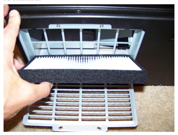
STEP 4: Install the new filter, replace the filter cover and insert the 2 screws.
