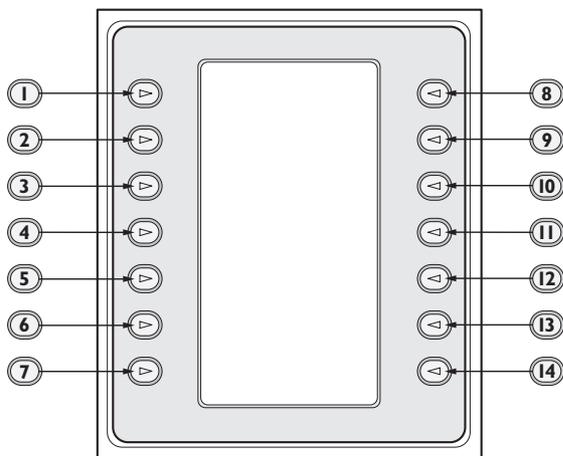
FIGURE 1-1 Softkey Numbering Guide
