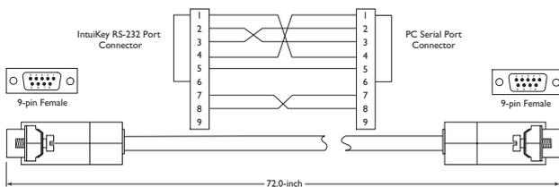
FIGURE 2-8 S1385 Cable Pinout
