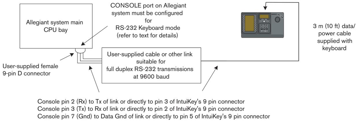
FIGURE 2-5: Direct Connection to Allegiant's Console/Printer Port
