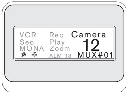
FIGURE 6-1 Status Display in System4 Mode
