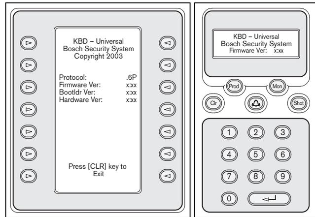
FIGURE 2-3 Initial Power-up Display
