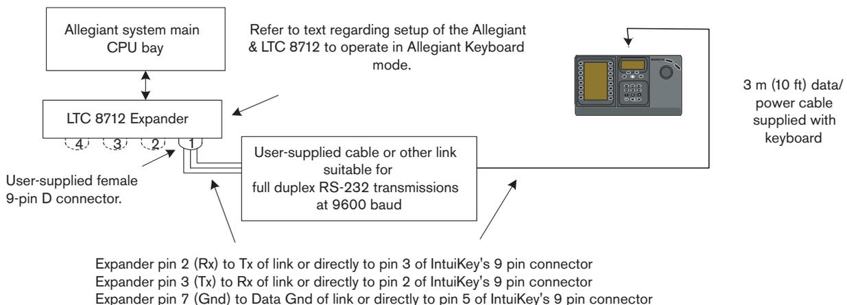
FIGURE 2-6: Configuration using LTC 8712 Series Console Port Expander
