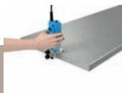
Both short ends of Encore worksurfaces are factory edged. On occasion a design will call for the installer to re-edge the product on site. The operation is simple and produces ar excellent inconspicuous end cap. However, it is much easier to complete a short end cap return on a workbench before the worktop is screwed in place.
