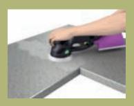
Ensure the sander is moved constantly during sanding operations. Holding the sander in one place can generate heat and create a depression in the worksurface. Ensure the worksurface is wiped clean between each sanding operation to remove debris and crif
