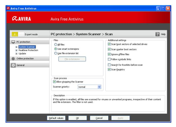
The Configuration opens a dialog box: You can save your configuration settings via the **OK** or **Apply** buttons, delete your settings by clicking the Cancel button or restore your default configuration settings using the **Default values** button. You can select individual configuration sections in the left-hand navigation bar.
