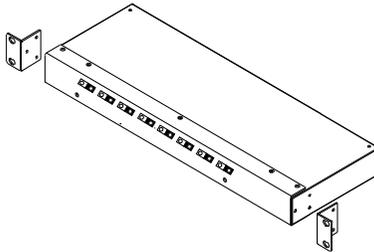
3. Slide the unit into the rack and secure it to the rack.
