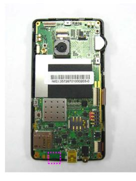
Connect the LCM FPC by a pair of tweezers and close its connector by plastic blade.
