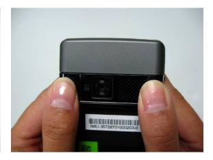
■ Step 16 Place the battery back and install the battery cover.
