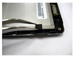
Install the keypad and arrange the keypad properly in the front cover.
