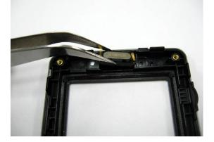
Step 2 Install the LCM on the front cover and place two top bezel rubbers to fix the LCM.
