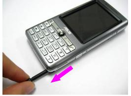
Step 2Remove the battery case and take the battery away.
