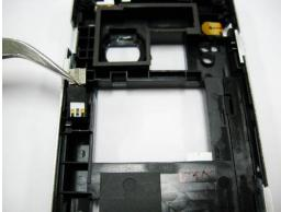
Release the antenna FPC by a pair of tweezers. Then tear off the antenna FPC from middle cover by hand.
