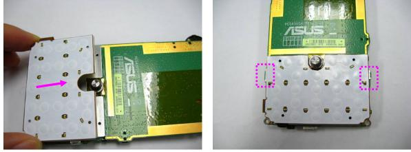
Connect the keypad FPC with main board by a pair of tweezers and close the connector by plastic blade.
