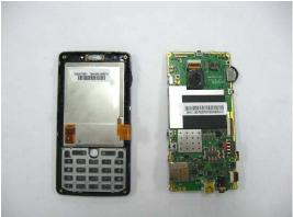
Open the camera connector by plastic blade and remove it from main board by hand.
