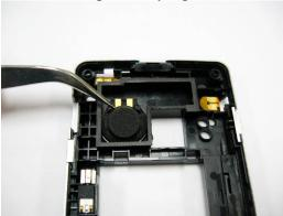
Step 7 Remove the vibrator by a pair of tweezers.
