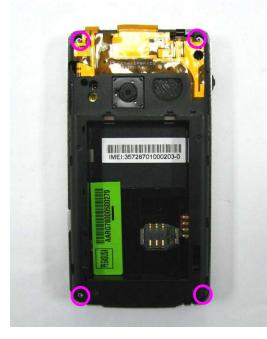
■ Step 15 Install the antenna cover and press to fix it.
