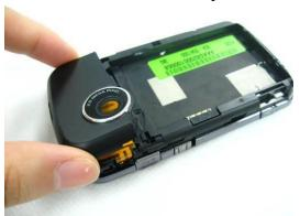
■ Step 16 Place the battery back and install the battery cover.
