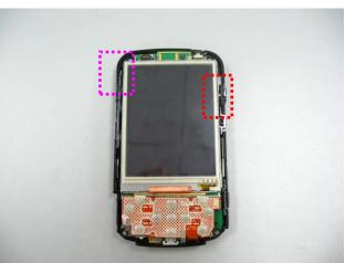
■ Step 11 Install the receiver by a pair of tweezers.
