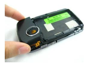
■ Step 4 Unscrew and remove 5 screws on PDA by screw driver.
