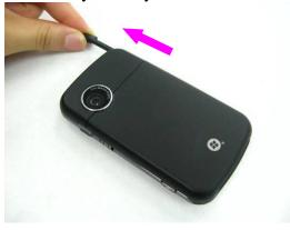
■ Step 2 Remove the battery cover and take the battery away.
