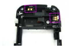
■ Step 2 Install the speaker on bottom case assy.
