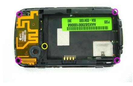
■ Step 15 Install the antenna cover and press to fix it.
