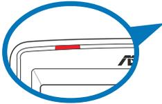
**NOTE** The charging status LED shows a steady red light as battery is being charged and steady green when battery is fully charged.
