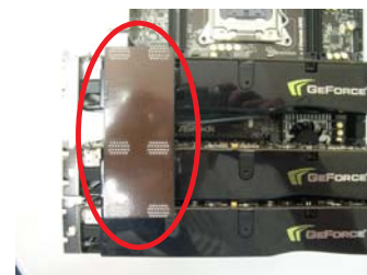
ASRock 3-Way SLI-2S1S Bridge Card
