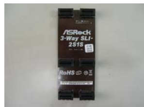
ASRock 3-Way SLI-2S1S Bridge Card
