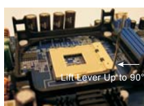
STEP 1: Lift The Socket Lever Up to 90°
