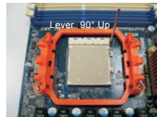
STEP 1: Lift Up The Socket Lever
