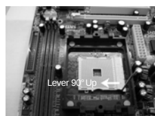
STEP 1: Lift Up The Socket Lever
