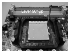
STEP 1: Lift Up The Socket Lever
