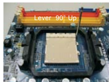
STEP 1: Lift Up The Socket Lever
