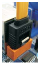
Connect the SATA data cable to the eSATAII connector (eSATAII_TOP)
