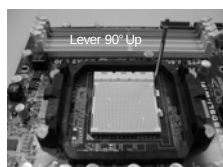
STEP 1: Lift Up The Socket Lever
