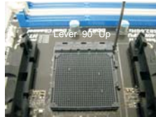
STEP 1: Lift Up The Socket Lever
