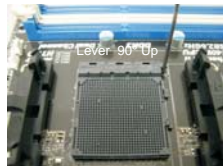
STEP 1: Lift Up The Socket Lever
