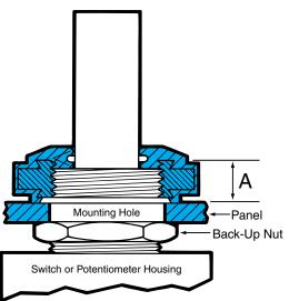
For proper installation of these boots, follow these five sequential steps. It is EXTREMELY IMPORTANT that the number of threads on the switch/potentiometer bushing EXPOSED ABOVE THE FRONT PANEL SURFACE be within the recommendation (see chart above). Failure to respect these maximums may result in boot damage (such as tearing).
