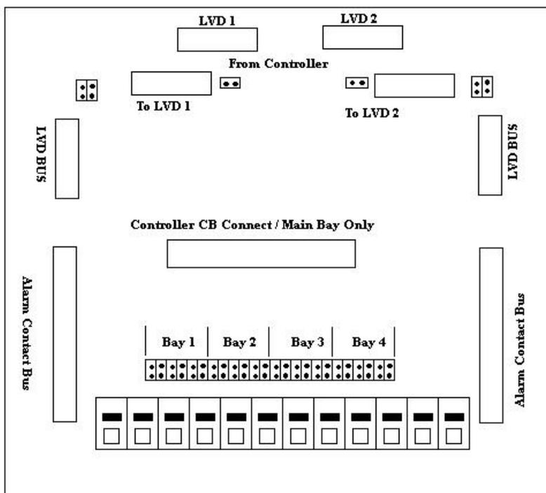
Figure 3.2-5 Circuit Breaker / LVD Expansion Board
