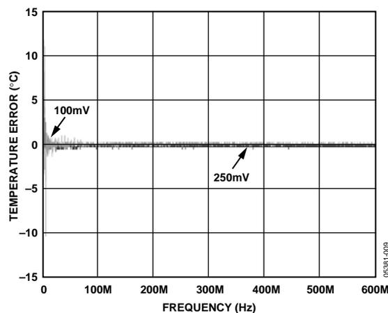
Figure 9. Internal Temperature Error vs. Power Supply
