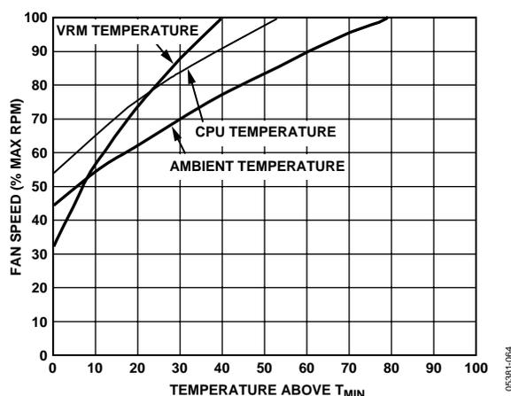
Figure 58. T<sub>RANGE</sub> and % Fan Speed Slopes for VRM, Ambient, and CPU Temperature Channels
