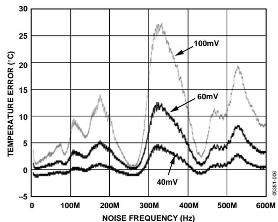
Figure 6. Remote Temperature Error vs. Common-Mode Noise Frequency
