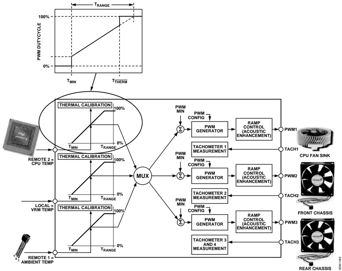
Figure 59. How  $T_{THERM}$  Relates to Automatic Fan Control
