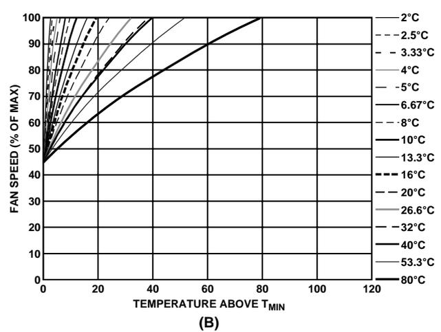
Figure 57.  $T_{RANGE}$  and % Fan Speed Slopes with  $PWM_{MIN} = 20\%$
