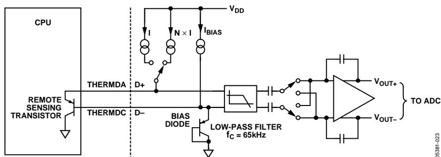
Figure 21. Signal Conditioning for Remote Diode Temperature Sensors
