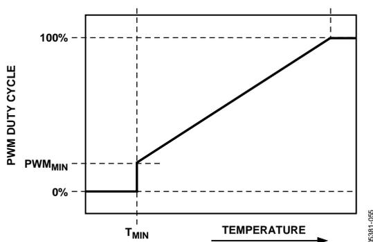
Figure 49. PWM<sub>MIN</sub> Determines Minimum PWM Duty Cycle
