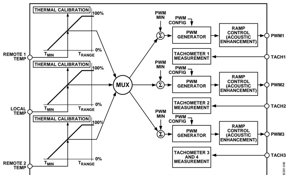
Figure 42. Automatic Fan Control Block Diagram
