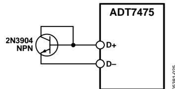
Figure 22. Measuring Temperature Using an NPN Transistor
