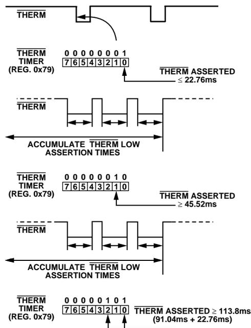
Figure 28. Understanding the  $\overline{\text{THERM}}$  Timer
