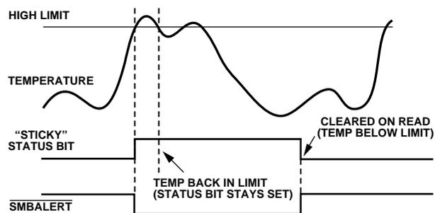
Figure 25.  $\overline{\text{SMBALERT}}$  and Status Bit Behavior
