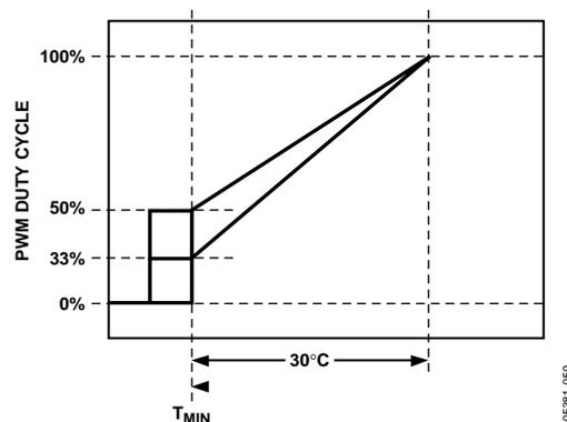
Figure 53. Adjusting  $PWM_{MIN}$  Changes the Automatic Fan Control Slope
