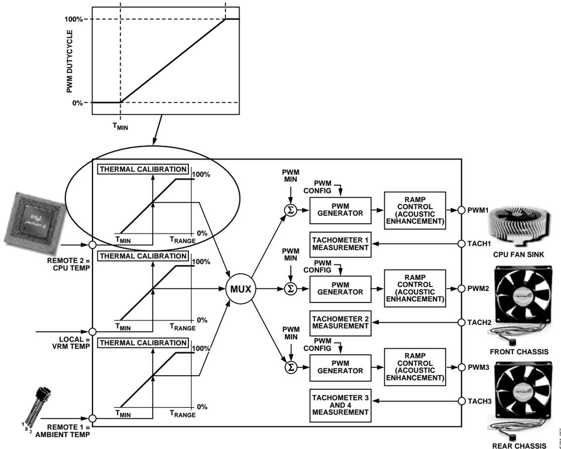
Figure 48. Understanding the  $T_{MIN}$  Parameter
