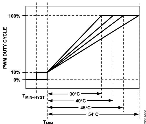
Figure 54. Increasing  $T_{\text{RANGE}}$  Changes the AFC Slope
