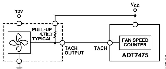
Figure 36. Fan with TACH Pull-Up to V<sub>CC</sub>
