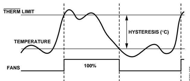
Figure 24.  $\overline{\text{THERM}}$  Temperature Limit Operation
