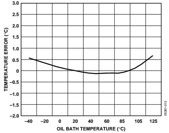
Figure 12. Remote Temperature Error vs. ADT7475 Temperature
