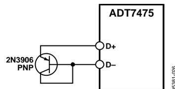
Figure 23. Measuring Temperature Using a PNP Transistor
