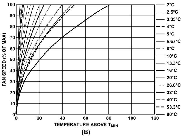
Figure 56.  $T_{RANGE}$  vs. Actual Fan Speed (not PWM drive) Profile
