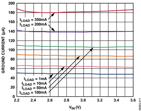
Figure 11. Ground Current vs. Input Voltage
