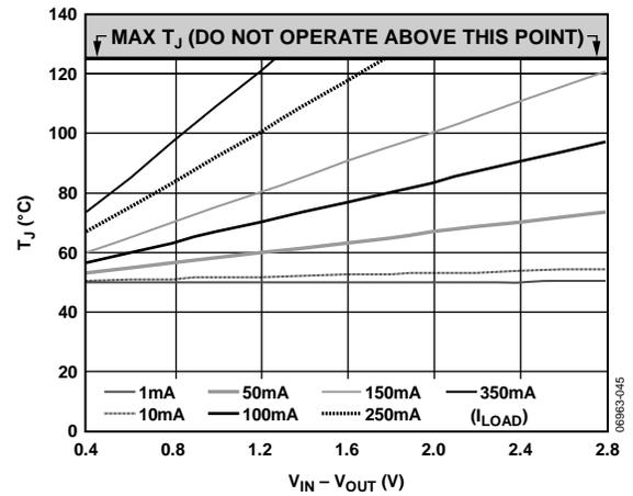
Figure 45. 0 mm<sup>2</sup> of PCB Copper,  $T_A = 50^\circ\text{C}$ , TSOT
