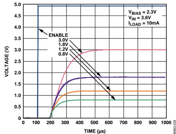
Figure 39. Typical Start-Up Time for Various Output Voltages
