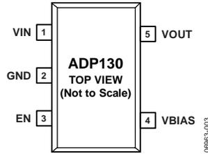
Figure 3. Pin Configuration
