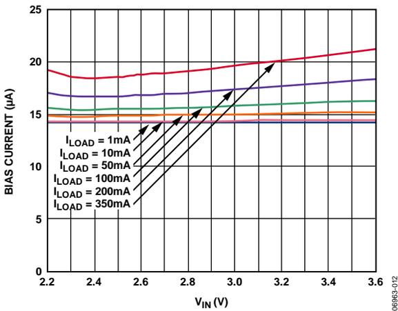
Figure 12. Bias Current vs. Input Voltage
