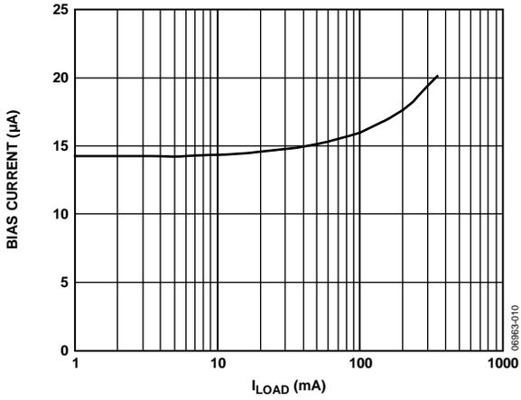
Figure 10. Bias Current vs. Load Current
