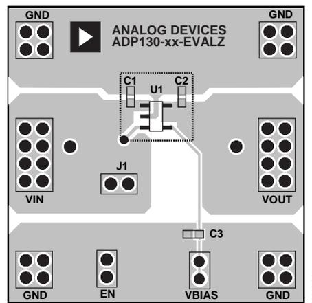
Figure 47. Example TSOT PCB Layout
