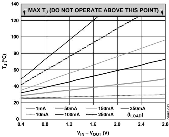
Figure 42. 0 mm<sup>2</sup> of PCB Copper,  $T_A = 25^\circ\text{C}$ , TSOT
