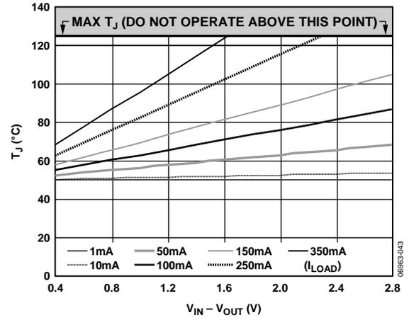
Figure 43. 500 mm<sup>2</sup> of PCB Copper,  $T_A = 50^\circ\text{C}$ , TSOT
