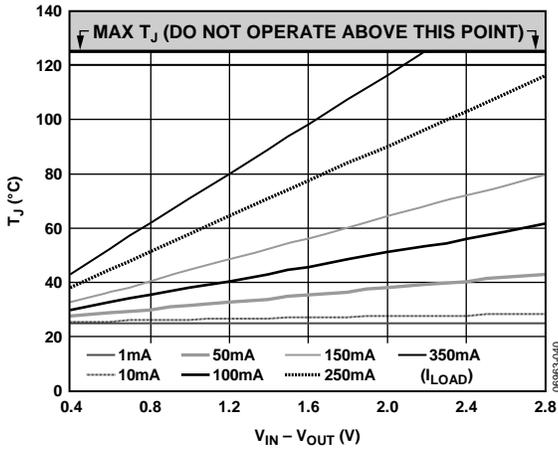
Figure 40. 500 mm<sup>2</sup> of PCB Copper,  $T_A = 25^\circ\text{C}$ , TSOT
