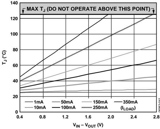
Figure 41. 100 mm<sup>2</sup> of PCB Copper,  $T_A = 25^\circ\text{C}$ , TSOT
