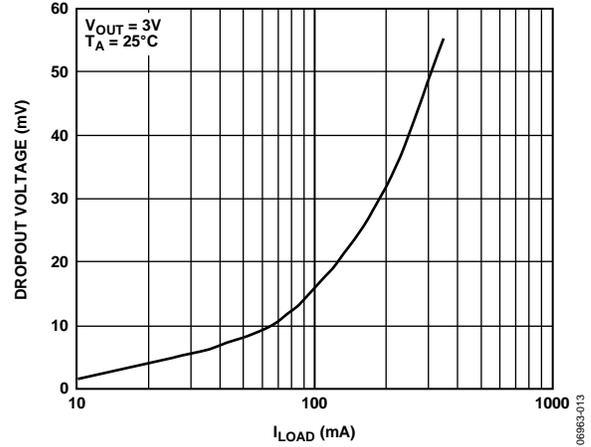
Figure 13. Dropout Voltage vs. Load Current,  $V_{OUT} = 3 V$
