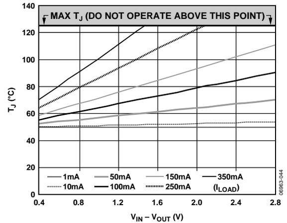
Figure 44. 100 mm<sup>2</sup> of PCB Copper,  $T_A = 50^\circ\text{C}$ , TSOT
