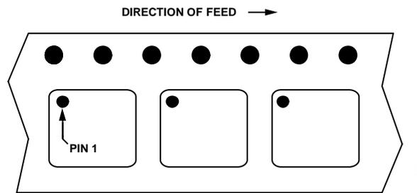
Figure 12. Microphone Orientation in Tape Until Date Code 1213
