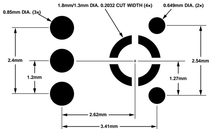
Figure 5. Suggested Solder Paste Stencil Pattern Layout
