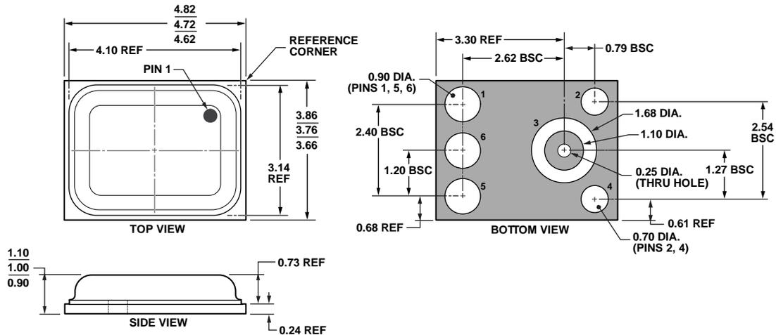
Figure 11. 6-Terminal Chip Array Small Outline No Lead Cavity [LGA\_CAV]
