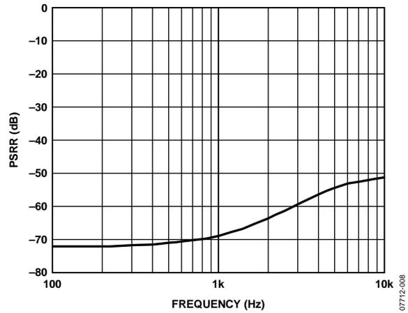
Figure 8. Typical Power Supply Rejection Ratio vs. Frequency
