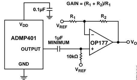
Figure 10. ADMP401 Connected to the [OP177](#) Op Amp
