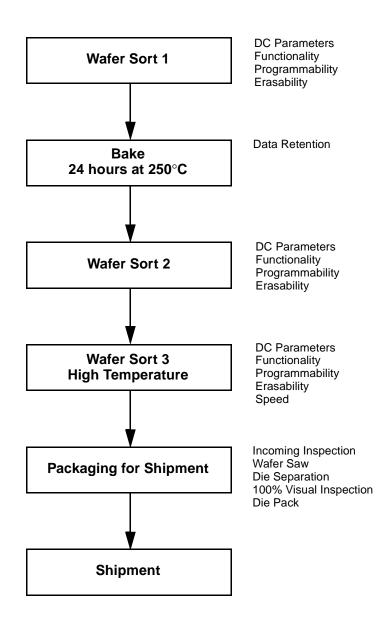
Figure 1. AMD KGD Product Test Flow
