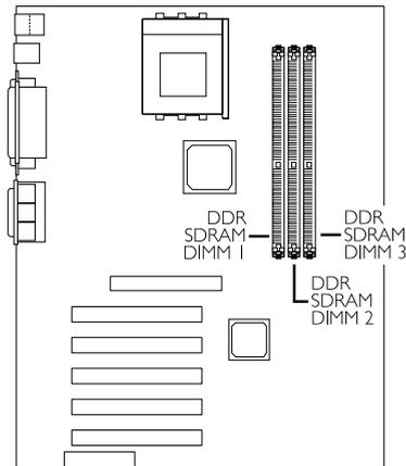
The system board is equipped with three 184-pin DDR SDRAM DIMM (Dual In-line Memory Module) sockets that support 2.5V DDR SDRAM DIMM. Double Data Rate SDRAM (DDR SDRAM) is a type of SDRAM that doubles the data rate through reading and writing at both the rising and falling edge of each clock. This effectively doubles the speed of operation therefore providing two times faster data transfer.
