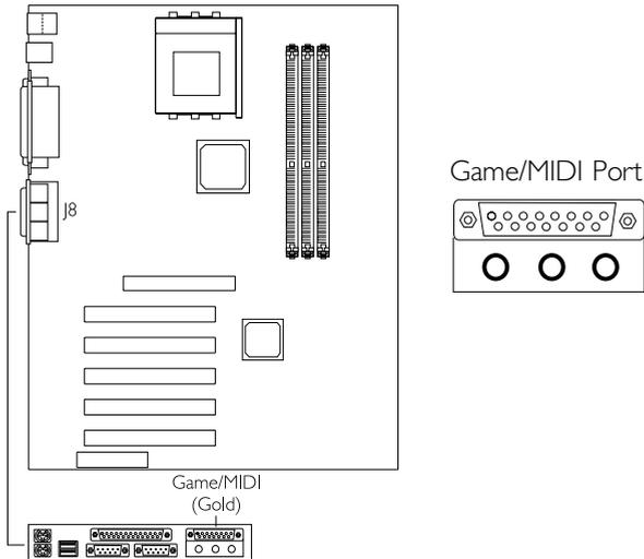
The Game/MIDI port is identical to that of a standard PC game adapter or game I/O port. Connect an analog joystick to the 15-pin D-sub connector (J8 - Gold) located at the ATX double deck ports of the system board. This port works well with any application that is compatible with the standard PC joystick.
