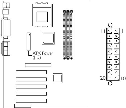
The pin assignment of the ATX power connector is shown below.
