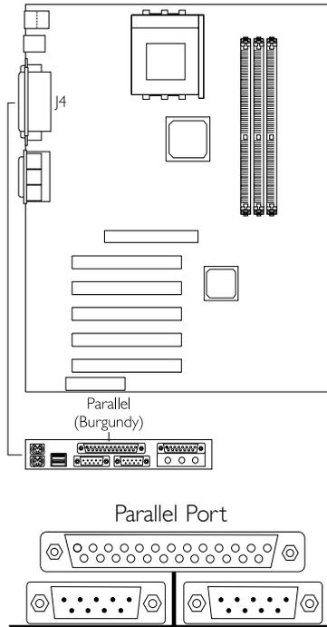
The system board has a standard parallel port (J4 - Burgundy) located at the ATX double deck ports of the board for interfacing your PC to a parallel printer. It supports SPP, ECP and EPP modes. You can set the port's mode in the Integrated Peripherals submenu ("Super IO Device" field) of the BIOS.
