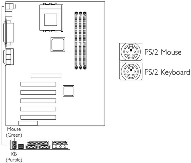
The system board is equipped with an onboard PS/2 mouse (Green) and PS/2 keyboard (Purple) ports - both at location J1 of the ATX double deck ports of the system board. The PS/2 mouse port uses IRQ12. If a mouse is not connected to this port, the system will reserve IRQ12 for other expansion cards.
