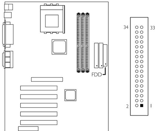
The system board is equipped with a shrouded floppy disk drive connector that supports two standard floppy disk drives. To prevent improper floppy cable installation, the shrouded floppy disk header has a keying mechanism. The 34-pin connector on the floppy cable can be placed into the header only if pin 1 of the connector is aligned with pin 1 of the header. You may enable or disable this function in the Integrated Peripherals submenu ("Super IO Device" field) of the BIOS.
