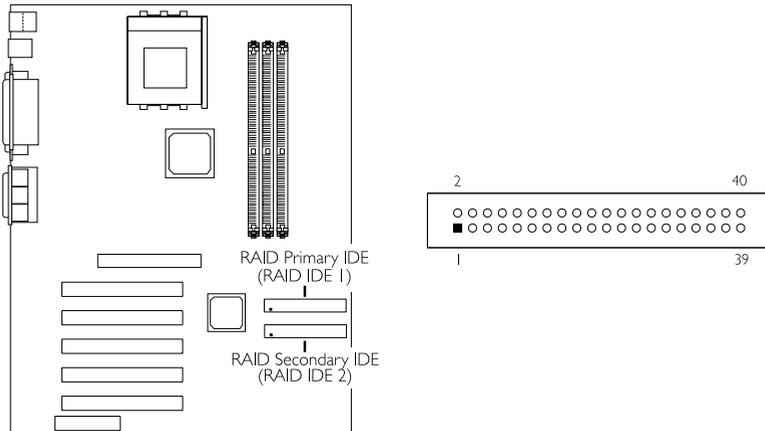
The system board is equipped with two shrouded RAID IDE headers that will interface four Enhanced IDE (Integrated Drive Electronics) disk drives. To prevent improper IDE cable installation, each shrouded RAID IDE header has a keying mechanism. The 40-pin connector on the IDE cable can be placed into the header only if pin 1 of the connector is aligned with pin 1 of the header. Use JP10 to enable or disable the RAID function.
