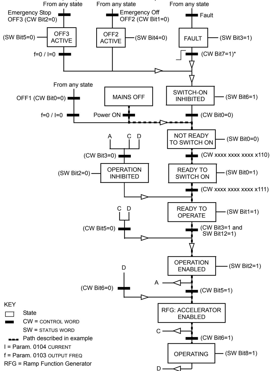
\*This state transition also occurs if the fault is reset from any other source (e.g. digital input).
