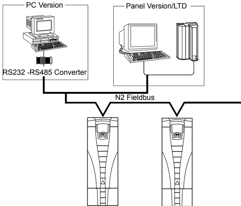
On the N2 Fieldbus each ACH550 drive can be accessed by the full complement of Metasys FMS features, including Change-of-State (COS) monitoring, alarm notification, scheduling, trend, and totalization.
