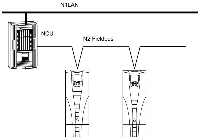
The following diagram shows the drives' integration to the Johnson Controls Metasys Companion system.
