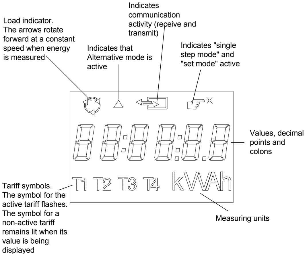
Fig. 2-5 DELTA single meter LCD
