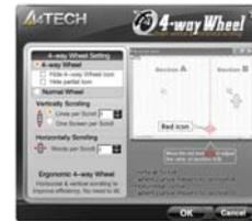
**A.** The 4-way Wheel is the latest scrolling technology. It splits working screen into 2 areas, A and B as shown. Depending on cursor position, the wheel will perform vertical or horizontal scrolling. For instance, when the cursor locates within A area, the wheel will perform vertical scrolling, and when the cursor locates within B area, the wheel will perform horizontal scrolling. It saves tremendous works instead of pulling the scrollbars, especially when working with Excel spreadsheet.
