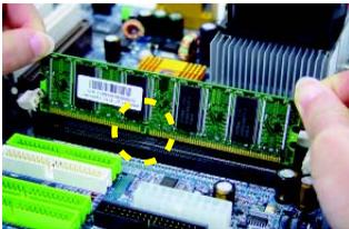
1. The DIMM socket has a notch, so the DIMM memory module can only fit in one direction.
