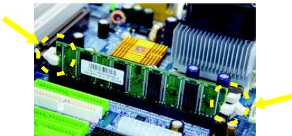
3. Close the plastic clip at both edges of the DIMM sockets to lock the DIMM module. Reverse the installation steps when you wish to remove the DIMM module.
