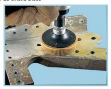
Remove paint, adhesive, weld burn, rust, heavy oxide and suface contaminants from large areas quickly and easily. No pressure required from the operator.  $\frac{1}{2} \int_{-\infty}^{\infty} \frac{1}{2} \left( \frac{1}{2} \int_{-\infty}^{\infty} \frac{1}{2} \left($
