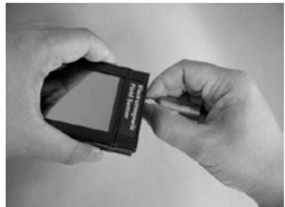
4. Insert and screw in the antenna making sure that it's not too tight or too loose. Do not use any tools other than your hand.
