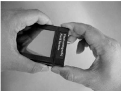
3. Press the sensor head firmly against the body until both surfaces are flat with each other.
