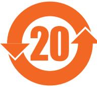
**This symbol, per Marking for the Control of Pollution Caused by Electronic Information Products, SJ/T11364-2006,**
