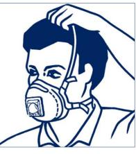
2. Place the top elastic strap around the head. above the ears. Untwist the strap.
