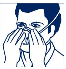
6. The seal of the respirator on the face should be fitchecked prior to wearing in the work area. a) Cover the front of the respirator with both hands, being careful not to disturb the position of the respirator. b) Inhale sharply. A negative pressure should be felt inside respirator. If any leakage is detected, adjust position of respirator and/or tension of strap. Retest the seal. Repeat the procedure until the respirator is sealed properly.
