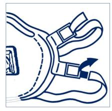
1. Thread top elastic strap through top buckles. Repeat for bottom strap and buckles. Place the bottom elastic strap around the head just below the ears. Untwist the strap.
