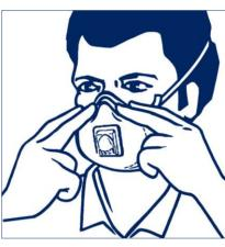
4. Using both hands, mould metal nosepiece comfortably to shape of nose.
