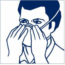
5. The seal of the respirator on the face should be fit-checked prior to wearing in the work area. a) Cover the front of the respirator with both hands, being careful not to disturb the position of respirator. b) Exhale sharply. A positive pressure should be felt inside the respirator. If any leakage is detected, adjust position of respirator and/or tension of strap. Retest the seal. Repeat the procedure until the respirator is sealed properly.
