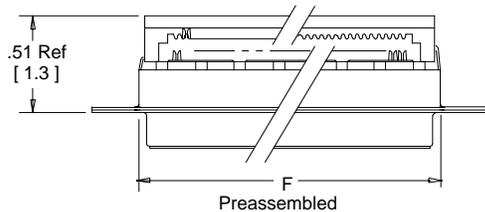
Note: Preassembled closed cover on Pin 1 side of connector.
