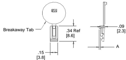
Note: #2216 B/A Scotchweld can be used to adhere keys.
