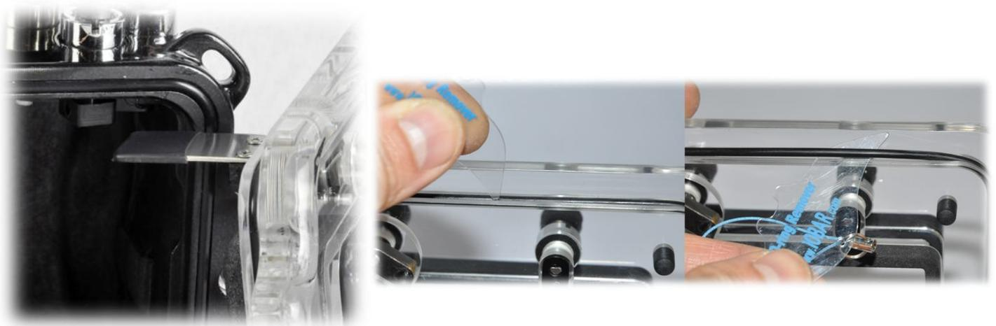
**The O-ring seal is the main barrier between the water outside and the air space within the camera. It is an effective barrier only if the seal is properly maintained. The O-ring seal should be inspected before every dive. The following information is provided for guidance in using and maintaining the O-ring seal.**
