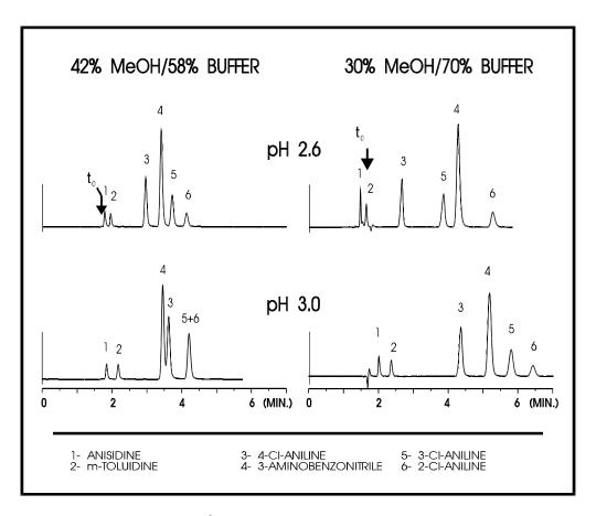
Zorbax® SB-CN, 4.6 x 150 mm (883975.905) 25 mM phosphate buffer; 1.0 mL/min.; 22°C
